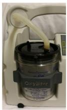
Remove the vacuum connection by twisting the tapered connector
