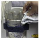
Push the tapered connector in to the female vacuum port, using a twisting action.
